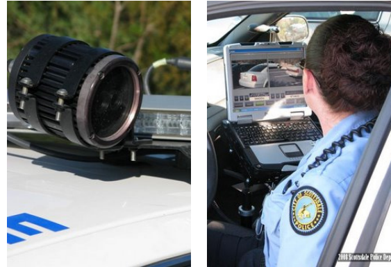
LPR camera and system
